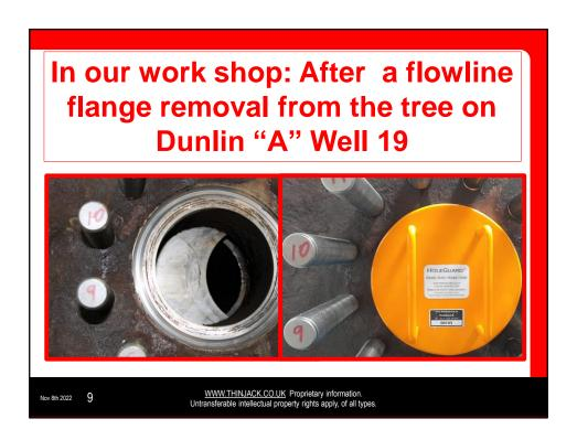
The flange removed, before placing HoleGuard, used our ThinJack service, with 200 tonnes of controlled force.
